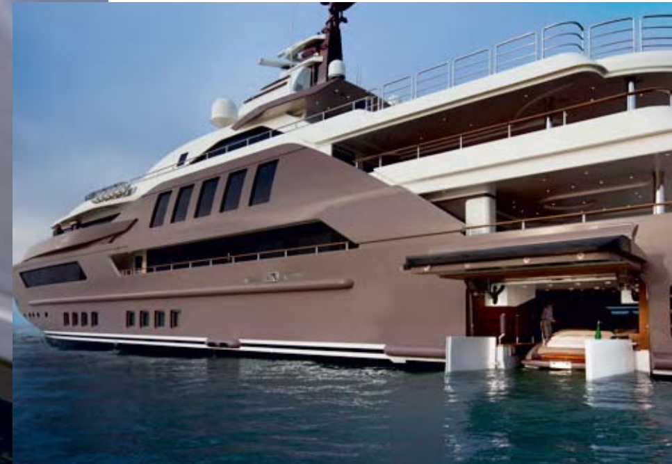
M/Y Jade 60 mt - Floodable garage Tender Bay concept
